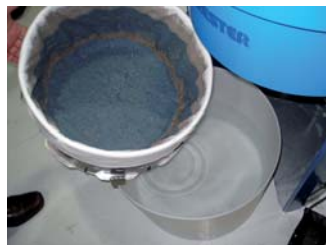
3. After 5 minutes paint particles will separate from the water and can be emptied into filter basket. The water can then be re-used and waste is reduced!
